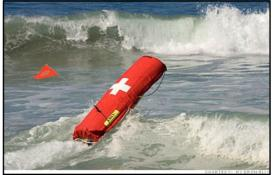
It can also patrol the water at a speed of five miles per hour for more than eight hours and weighs about 25 pounds. Compared to a human lifeguard, E.M.I.L.Y. can reach a drowning swimmer up to twelve times faster.
